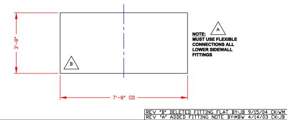
1. THIS IS A COMPUTER GENERATED DWG. DO NOT REVISE BY HAND. 2. DIMENSIONS WILL VARY ±3% DUE TO VARIATIONS IN MULTIPLE MOLDS & CONDITIONS PREVALENT DURING MANUFACTURE & USAGE. 3. NO GALLONAGE MARKERS THIS TANK.
