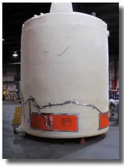
Poly Processing's tank heating systems are specifically designed for temperature maintenance of polyethylene tanks. SPX Tank Heating Systems maintain a desired product temperature, not to exceed 100 degrees F. Each heating system consists of tank heating pad(s) and a temperature controller.
