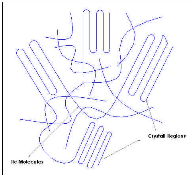
**Figure 1** Crystalline and amorphous regions in Polyethylene
